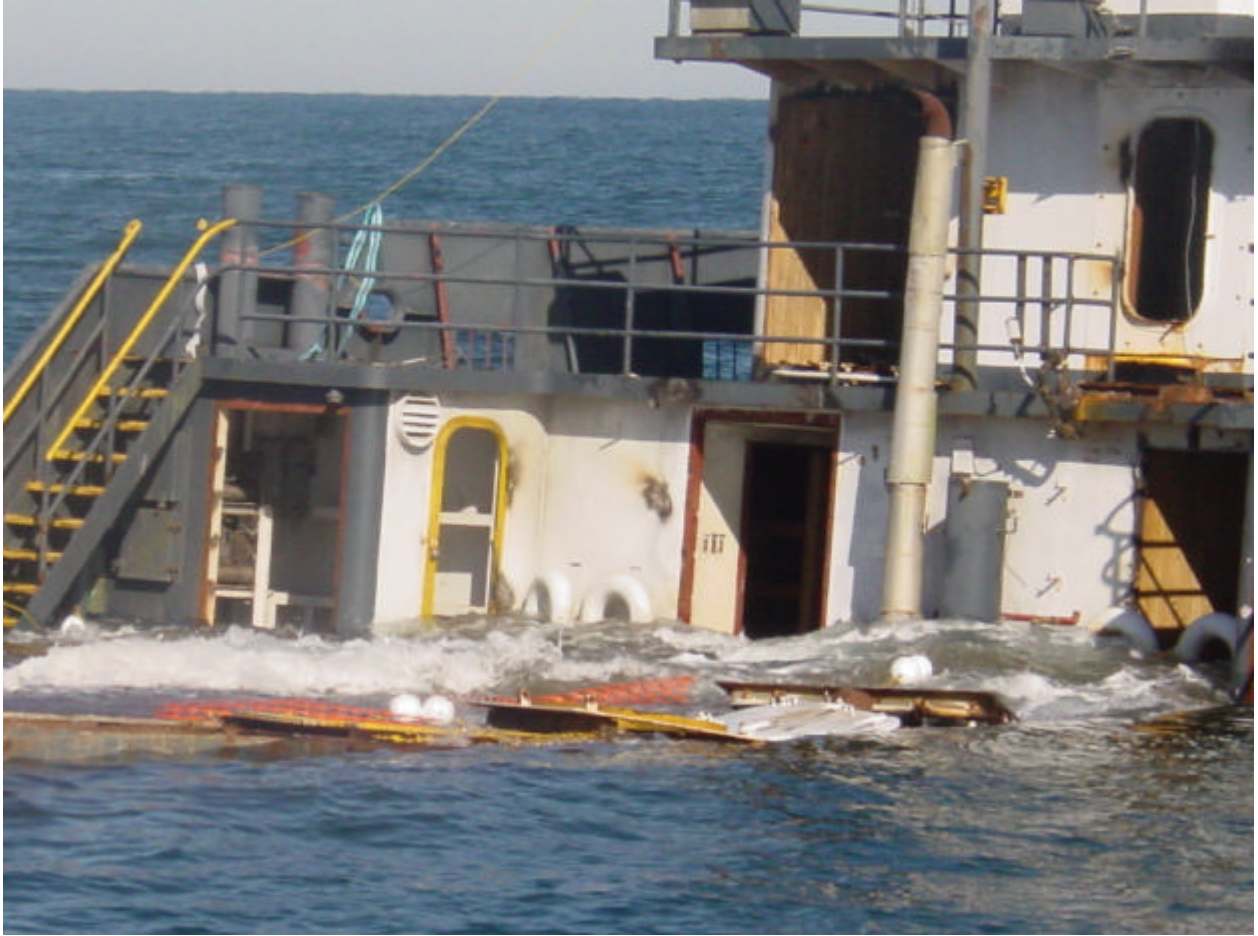
Water Rushing in on the Deck and in the Rooms.
